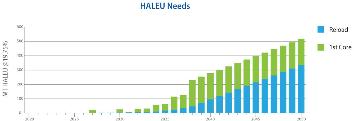
Figure 4. Projection of HALEU needs for advanced non-LWRs to 2050.
